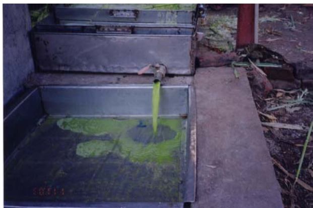
Extracted juice being strained into settling tank
